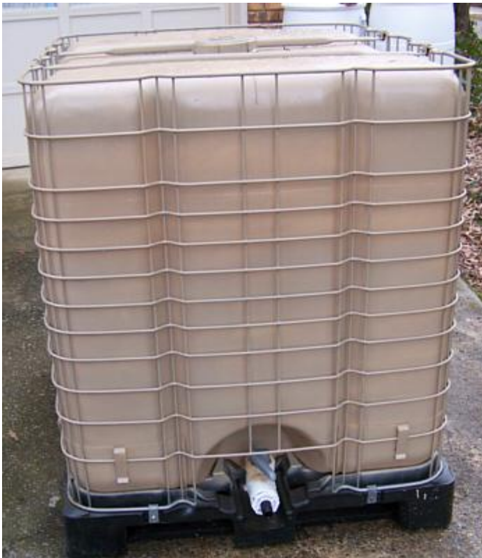
The tank after a coat of Krylon Fusion Satin Khaki paint.
